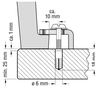
For a precise fit, the cut-out must be produced in the worktop by reference to the original sink. The supplied installation templates provide guidance here.
