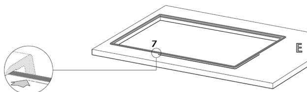
**F** Seal cleaned cut-out edge with silicon, fill
