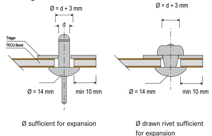
Connection of two or more metal parts joined together, drilled, and pierced by a rivet.
