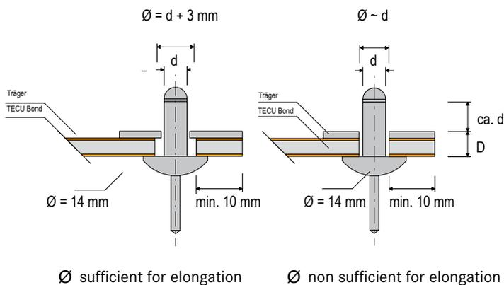
The forces at work on the TECU® Bond panel determine the type of rivet to be used and its diameter. Tearing out the rivet should be avoided. In rivet selection, it is recommended to apply a safety factor of 3 to the values specified by the supplier for tensile and shearing strengths. The rivet must be set in the middle free of constraint forces using a rivetting tool (see Figure above).
