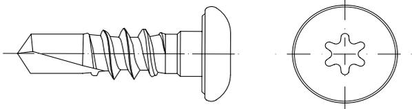
Screws must not be subject to additional bending by shearing forces on the structure elements. Screws must always be placed perpendicular to the surface.
