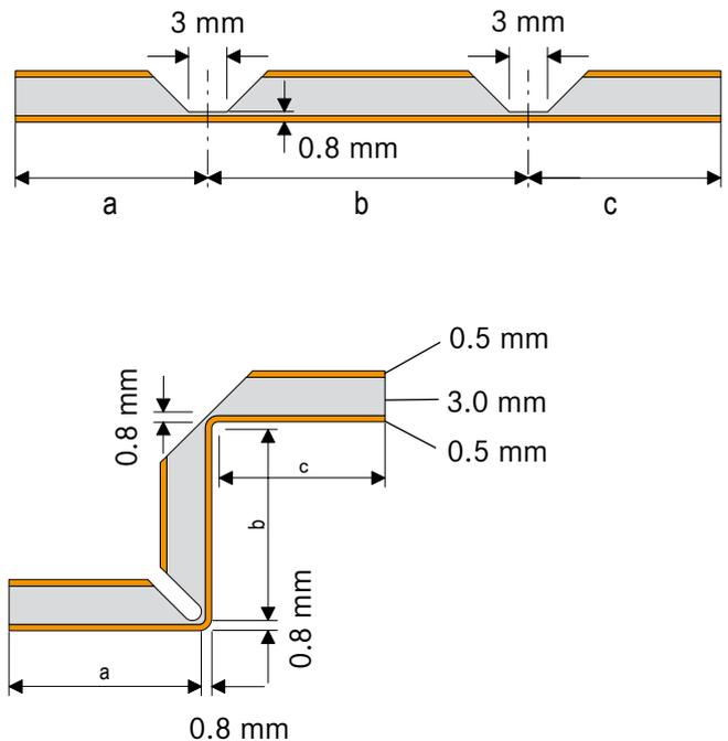
Fig. in- and exterior corner 90°
