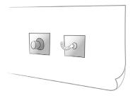
Sealing of through elements with sleeves/accessories
