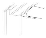
Correct jointing of wall-roof node
