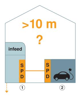
IEC 60364-4-44 requires surge protection. If none exists in the building, at least one type 2 SPD must be erected at the infeed point of the system during the creation of a new circuit.
