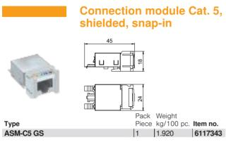
Connection module Cat. 5e shielded, with a RJ45 slot. Including an EMC screen hood, a dust cover, a cable tie, a snap-in fastening frame and mounting instructions. Suitable for installation in support plates, type MTM 2C and MTM 3C, mounting plate type MPR2 2C, mounting support type MTGE2 2C, MTGE2 15 2C and MTGE2 F 2C.
